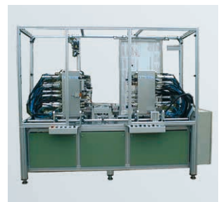
23 placing heads to assemble a computer chassis
