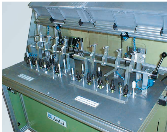
10 placing heads to assemble automotive sealing strips
